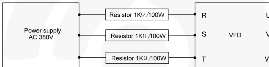
Figure 8-2 380V charging illustration of the driven device
